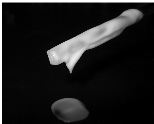
Figure 3. A glass rod was dipped into the gelatinized GB emulsion and shaken violently.
